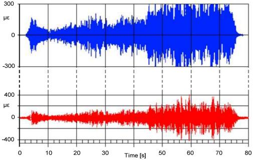
Fig. 6. Comparison of strain measured by EF (top) and electrical reference sensor (bottom).
