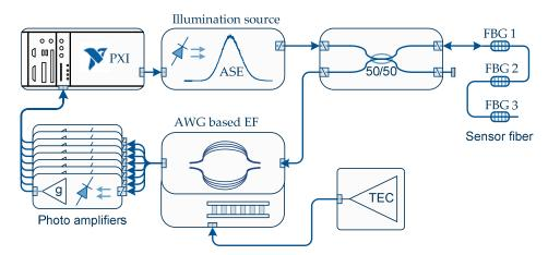
**Fig. 1.** EF interrogator. An autonomous spontaneous emission (ASE) light source illuminates the FBG sensors. Light that is reflected by the sensors is guided to an AWG configured as EF.
