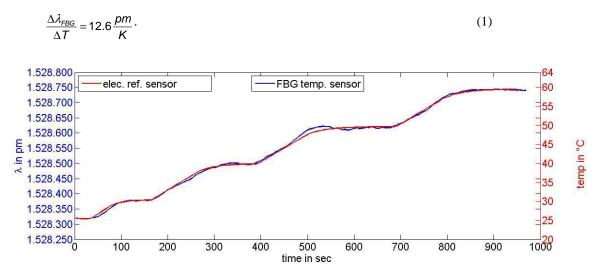
**Fig. 3.** An FBG configured as temperature sensor was read out with the SL interrogator. An electrical reference sensor confirms the measurement results.
