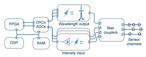
**Fig. 2.** SL interrogator. The output wavelength of the laser diode is controlled by three input currents generated by digital to analog converters (DAC). Intensities of light pulses that are reflected by a FBG sensor are measured and digitized. A centroid algorithm implemented in a digital signal processer (DSP) calculates the mean wavelength of the sensor.
