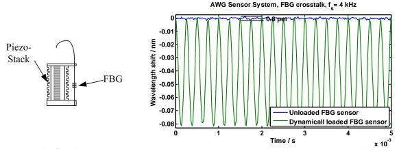
**Fig. 5.** Left: A vibration test stand was developed prior to the test in order to apply a dedicated frequency to a FBG sensor. Right: Measurement of a 4 kHz vibration using the EF interrogator.
