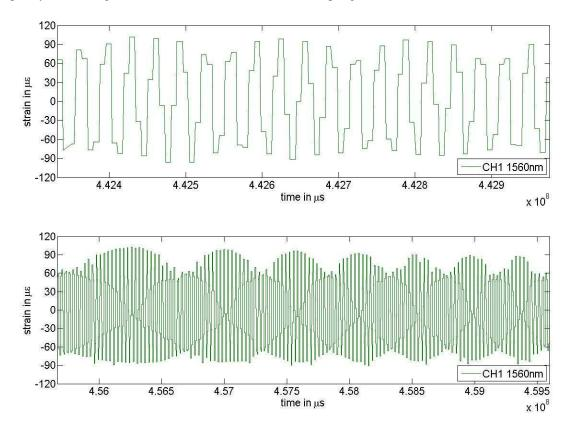
**Fig. 4.** One FBG sensor with a design wavelength of 1560 nm measured with the SL interrogator during frequency sweep of the structural demonstrator (top: 31 Hz excitation frequency). Vibration measurement shows beat frequencies due to under-sampling when the structure is excited with frequencies higher than 65 Hz (bottom).
