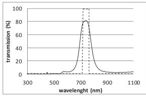
Figure-6. Ideal versus realistic optical bandpass filter characteristic.
