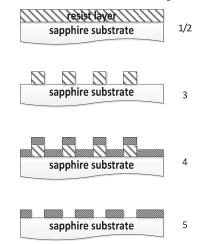
Figure-7. Schematic of the mesh filter production steps, the numbers correspond with the numbers in the text.
