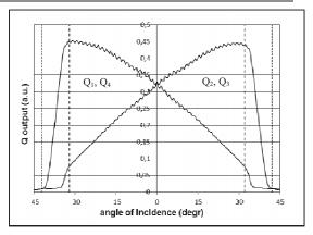
Figure-4. Quadrant signal as function of angle of incidence. The ripple on the signal is caused by the mesh filter. Vertical lines designate  $\pm 32^{\circ}$  and  $\pm 42^{\circ}$  respectively.
