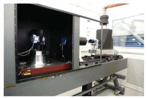
Figure-10. Test set-up for performance testing and calibration with solar simulator and FSS mounted on 2-axis rotation table.
