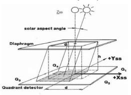
Figure-2. Quadrant sensor operation principle
