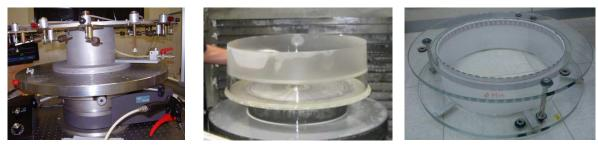
Fig. 2. A) Side view of the astatic support system used during OOR metrology. B) Raw quartz glass tube mounted on the grinding machine at the Heraeus Quarzglas facility. C) First shell integrated in its SSS. Proc. of SPIE Vol. 10565 105652N-5
