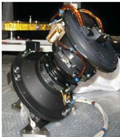
Fig. 7: GOCI Pointing Mechanism (w/o mirror)
