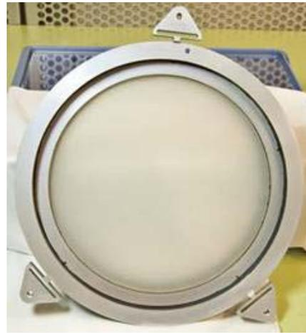
Fig. 12: Full pupil Solar Diffuser (external side)
