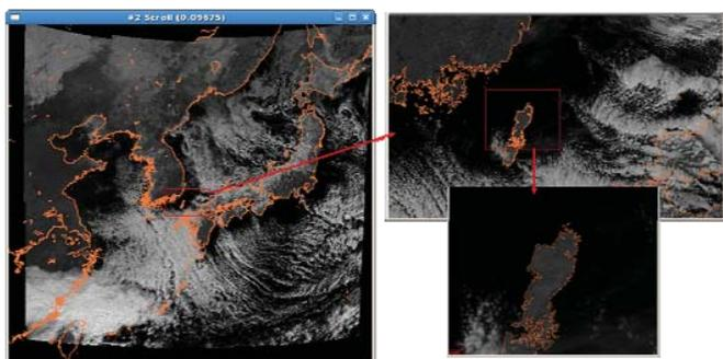
Fig. 20: Example of shore line matching on typical images shows good geo-localisation achieved by the Image Navigation & Registration SW on bands B7 & B8 (which provide best earth/water contrast)
