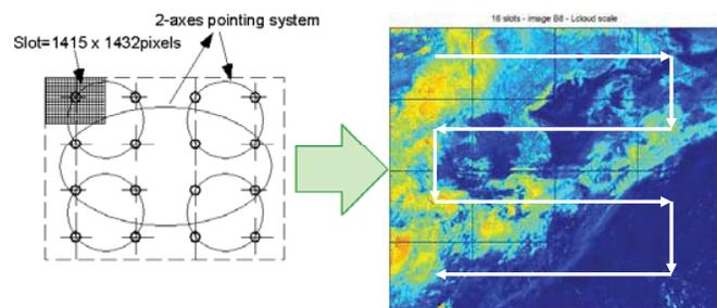
Fig. 5: Principle of GOCI image acquisition
