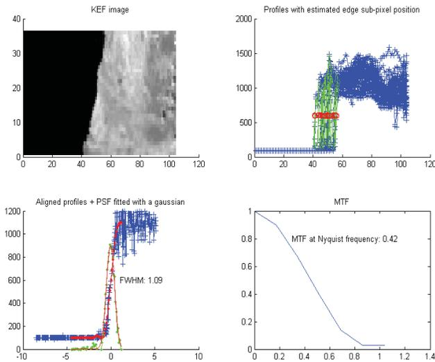
Fig. 14: example of MTF evaluation point on a transition edge within the GOCI image.
