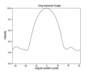
Figure 5 : long exposure image average of 1000 short exposure images during (~6 min)
