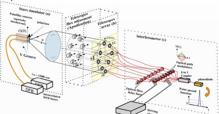
Fig 2 : General scheme of our Temporal hypertelescope (THT) test bench. The main sub systems are described in detail in the text: The star simulator, the telescope array and the combining interferometer. Proc. of SPIE Vol. 10565 105650E-3
