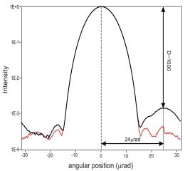
Figure 7 : Comparison between an unbalanced (dynamics ratio D= 1000) binary star image (in black line) and a single star image (in red dots)
