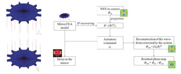
Fig. 1. Left: Finite Element Model of the MADRAS mirror (actuator are represented by springs, in red) - 63708 hexaedrical elements, 77979 nodes - Right: Method for design optimization, based on the finite element model's influence functions: the three minimized criterions are the stress in the mirror, the actuators commands and the residual wave-front error.
