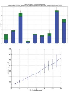
Fig. 7. System performance with dead actuators (FEA results): Top: comparison of the precision of correction of a system fully functionnal and a system with one dead actuator - Bottom: evolution of the mean expected residual wave-front with the number of dead actuator (each point is a statistic on 50 random sets of dead actuators and 100 random WFE for each set).
