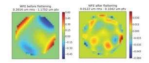
Fig. 9. WFE before and after flattening (tip, tilt and focus substracted).
