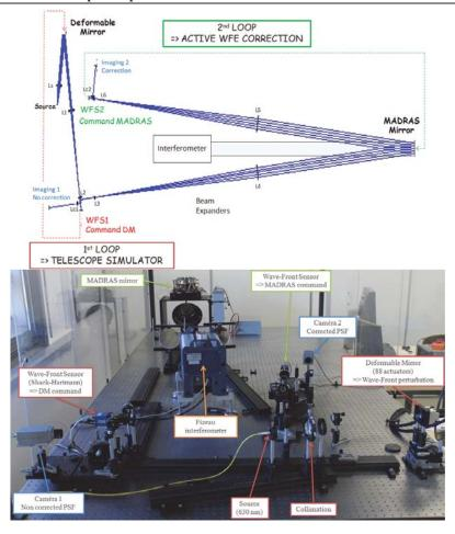
Fig. 8. MADRAS test-bed: optical design and picture.
