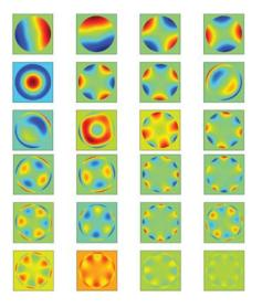
Fig. 5. System's Eigen Modes, sorted from the less to the more energetical, deduced from a Singular Value Decomposition of the measured IF base.
