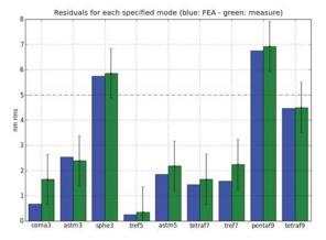
Fig. 6. Residual WFE computed for each specified modes, with simulated and measured IF (errorbars correspond to the interferometer precision:  $\pm$  1 nm).
