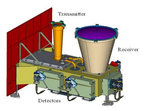
Fig. 1 LOLA Instrument Diagram
