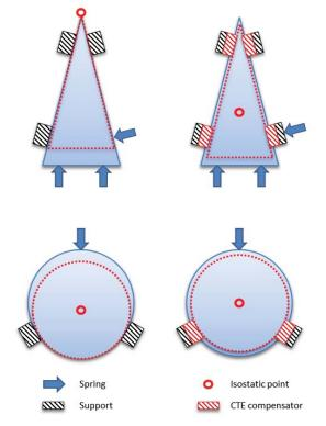
Figure 3: Isostatic points for various mounting methods of lenses and prisms. The circle indicates the location of the isostatic point The situation at operational temperatures is shown with the red dotted lines.
