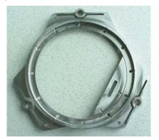
Figure 4: Kinematic mount with 3 double ended clamped leaf springs at 120 degrees each at the circumference, for accurate a-thermal alignment. The three centrally located dowel pins are key for the alignment accuracy of this kinematic mount
