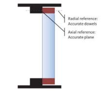
Due to the decrease in manufacturing accuracy of the large diameters the accurate fit solution turns out to be less accurate. The table shows final positional accuracy with a precise but normal manufacturing strategy.
