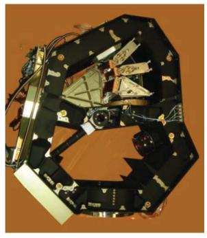
Figure 15: X-shooter near IR Spectrograph
