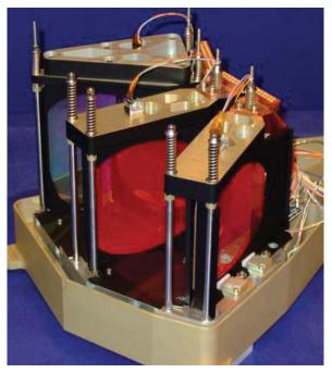
Figure 14: The X-shooter prism bench. The fully integrated prism with bench with the spring loaded top supports. The special CTE compensation pads (white) are seen at the side of the prism.
