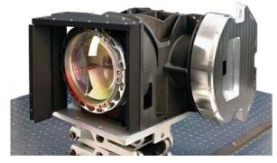
Figure 8: 2K camera assembly; at the front the triplet assembly, the doublet is located inside the camera structure (at the right hand side) and thus not visible in the photo.
