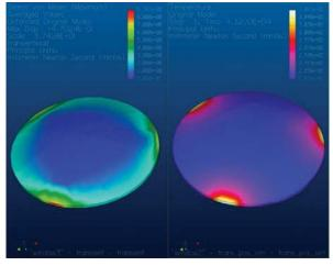
Figure 5: Thermo elastic analysis of the SPIFFI L1 lens. Left the maximum von Mises stresses of 8.2 N/mm2 due to the temperature gradient of 18 K (right) caused by a cool down rate of 24 W/h. cooling input at three spots at the lens circumference.
