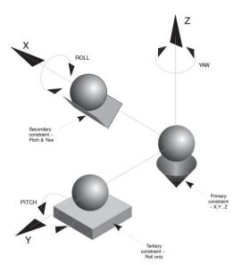
Figure 1: The theoretical representation of the classical "cone, groove and flat" kinematic mount (figure: courtesy Newport Corp.). The three balls are part of the element. With this type of mounting extra precautions are necessary to ensure correct positioning of all parts e.g. under varying gravity orientation. That makes this type of mounting less suitable for many astronomical applications (instruments in cassegrain foci, space instruments).
