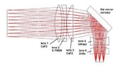
Figure 9: Optical design of the SPIFFI 2K camera consisting of 5 lenses and one folding flat. The lens triplet consists of the first three lenses while the last two lenses are joined in the doublet.
