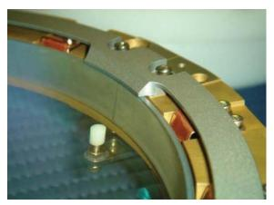
Figure 6: X-shooter corrector lens with additional thermal leads; the copper strips at the lens circumference
