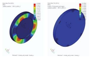
Figure 8: Stress distribution within the total assembly (left) and the lens (right).
