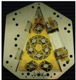
Figure 13: The X-shooter test prism base support plate. Clearly visible are the special thermal contact pads and their elaborate spring connections that ensure thermal contact with the prism at all times. On the pads the small circles of indium foil to improve thermal conductivity. The Kapton layer between prism and support pads reduces friction for maximum compensation during cool-down/warm-up. CTE compensation pads are located on either side of the prism area.
