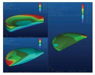
Figure 7: Additional expected lens deformation due to CTE uncertainties within SPIFFI; L1 1.4 nm (lower left), L2 1.9 nm (upper left) and L3 (right)8.3 nm at an operational temperature of 77K.
