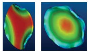
Figure 2: Deformation of a lens (SPIFFI L1) with 3 and 6 pads. The total force is identical for both situations but divided over respectively 3 or 6 points, resulting in a surface deformation of L1 of respectively 3.83 nm and 2.04 nm. The 6 mounting pads show less deformation 2.04 nm, compared to 3.83 nm for three pads, and in addition a much favourable surface shape
