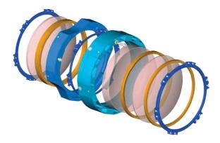
Figure 10: The main housings of the triplet are accurately lapped to the required dimensions. The axial springs push the lenses (transparent) to the axial supports (darkest colored rings) that are referenced to these outside (lapped) surfaces. The aluminium contact surfaces with the lenses are treated by Teflon-filled hard anodization to reduce internal friction. Within the housing the six radial supports are located (small light grey circles).
