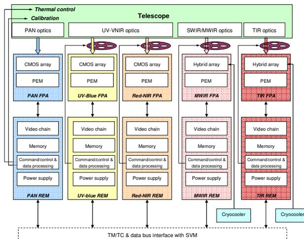
Fig. 9. Electrical architecture of the instrument
