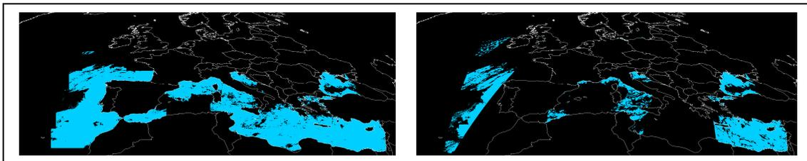
Fig. 2. Ground coverage within one day for Geo-Oculus (left) and LEO (Sentinel 3, right) are highlighted blue
