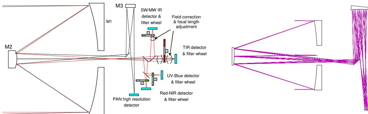
Fig. 6. Optical configuration (left: synoptic, right: PAN channel)
