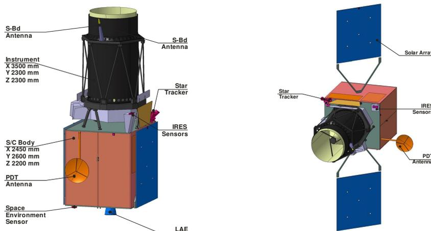
Fig. 4. Geo-Oculus spacecraft configuration (left: stowed, right: deployed)
