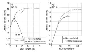
Fig. 5. Pre- and post- irradiation cut-back measurements performed for "NP-Si+" and "NP-Al" fibers.
