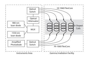
Fig. 2. Irradiation Set-up
