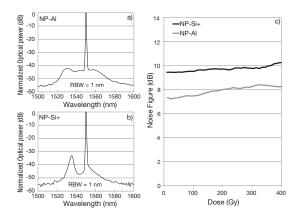
Signal + ASE spectra and Noise Factor evolution as a function of the dose deposit. The spectra were obtained at 1 nm Resolution Bandwidth (RBW).
