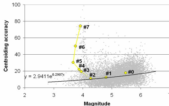
Fig 9 Centroiding as a function of magnitude (for LCMS based camera in MABS) (#n indicates the number of detector pixels which are saturated in a 4 x 4 interpolation frame)
