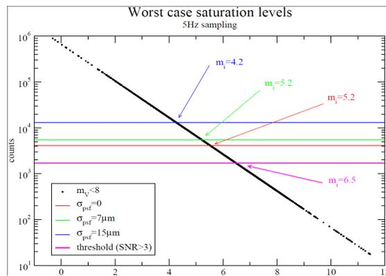
Fig 8 Dynamic range calculations for LCMS based camera in MABS
