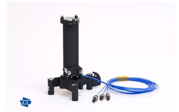
**Fig. 5** The WFS qualification model. The WFS's exterior is black for stray light reasons. The interface to the SiC GAIA-focal plane is by 3 tangential invar flexures. Three calibration fibres can be seen (blue). The WFS is 150 mm high, and weighs less then 500 grams.
