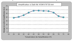
Fig. 13 : energy level at the output of the additional amplifier for an incident pulse of 26mJ
