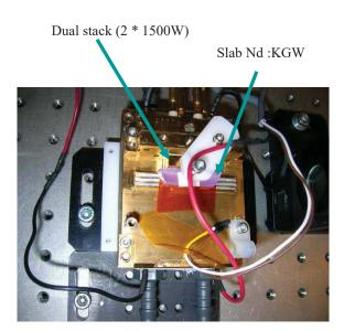
Fig. 12: design of the additional amplifier for SAGE
