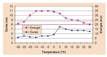
Fig. 6. Energy and pulse duration versus temperature
