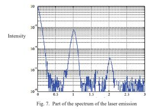
Using an appropriate direct detection system, LATMOS showed that it could be possible to use this laser as a luminous source for a Doppler Lidar despite its high spectral multimodality. Most of the existing Doppler Lidars require a longitudinally monomode laser source. The lidar we aim to build would work with the ChemCam multimode laser, much simpler to develop than a monomode laser requiring the injection of a stable frequency and a servo-loop for stabilization of the laser on this frequency.
