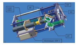
Fig. 10 : View of the Doppler Lidar laboratory model developed at LATMOS
