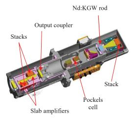
Fig.4. Optical design of the laser
