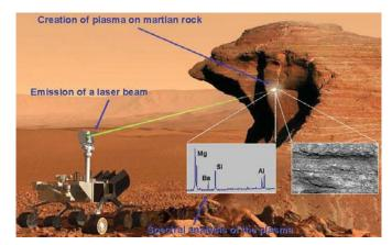
Fig.2. General principle of ChemCam
