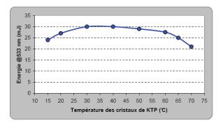
Fig. 14 b : energy at 533nm with two KTP crystals (length of 4 mm) for an input energy of 58mJ at 1067nm
