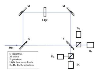
Fig.8 : detection system of the Doppler Lidar (Mach-Zehnder interferometer)
