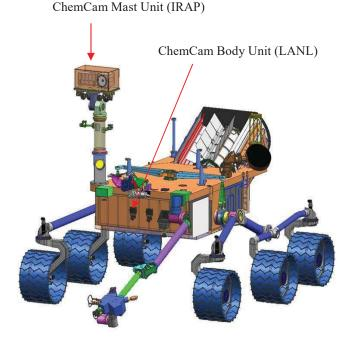
Fig.1. View of MSL Rover and situation of ChemCam (copyright NASA)
