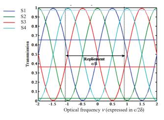
Fig.9 : transmission of the 4 channels (S1, S2, S3 and S4) with respect to
