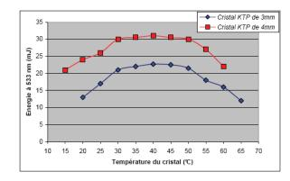
Fig. 14 a : energy at 533nm with one KTP crystal (length of 3mm and 4mm) for an input energy of 58mJ at 1067nm
