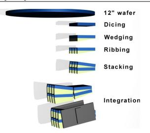
Fig. 4. Illustration of the process steps for manufacturing a SPO mirror module.
