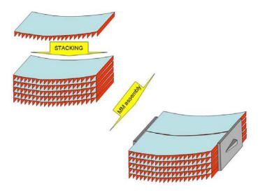
**Fig. 1.** Illustration of the Silicon Pore Optics technology. Several curved mirror plates are stacked by direct bonding of the silicon surfaces. Pores inside the mirror plates allow the X-rays to pass through the optics. Two SPO stacks are connected by brackets to form a mirror module for focusing X-rays by two reflections.
