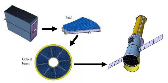
Fig. 2. Illustration of the modular approach for the IXO telescope. About 200 SPO mirror modules are integrated into a petal and eight petals are integrated on an optical bench of the spacecraft.
