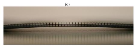
Fig. 5. (a) SPO stack of coated mirror plates
