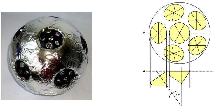
**Fig. 1a)** Test target sphere containing 12 RR arrays
