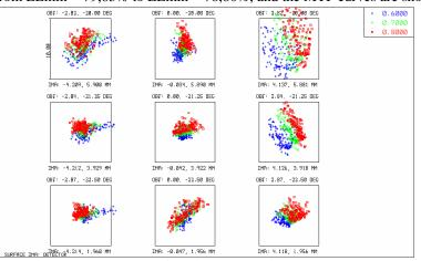
Fig. 9. Spot Diagrams of the Stereo Camera of BepiColombo mission at  $T_f = -20^{\circ}$ C: kinematic constraints
