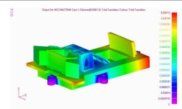
Fig. 5. Results of thermo-elastic analysis from integration temperature  $T_i = 20^{\circ}C$  to temperature  $T_f = -20^{\circ}C$ .
