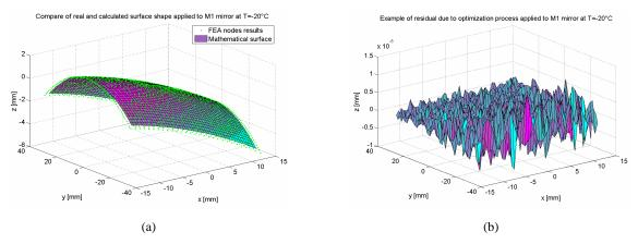
Fig. 6. Example of surface interpolation using Nonlinear Least Square algorithm applied to the shape of M1 mirror: (a) surface interpolation; (b) residuals.
