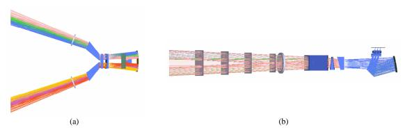
Fig. 1. Ray-trace scheme of the Stereo Camera of BepiColombo mission: (a) top view; (b) left view.
