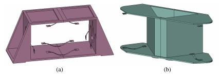
Fig. 3. Example of kinematic constraints applied to the housing systems of the lenses (a) and prisms (b).
