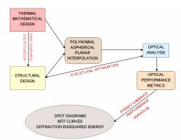
Fig. 4. Scheme of the method to study the changing in optical performance due to thermo-elastic analysis.
