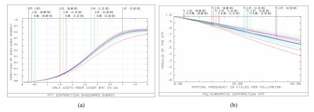
Fig. 10. Diffraction Ensquared Energy (a) and MTF curves (b) of the Stereo Camera of BepiColombo mission at  $T_f = -20^{\circ}C$ : kinematic constraints.
