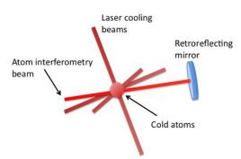
Fig. 1. Schematic view of the atom interferometer. The atoms are cooled down to  $10 \,\mu$ K. The cooling beams are then turned off for the interferometric measurement, so that the cold atom cloud is in free fall. The retroreflecting mirror defines the phase reference of the laser ruler.
