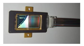
**Fig. 3.** SWIFTS 400-1000 mockup: A 1K frame transfer CCD is surrounded by a glass plate containing parallel waveguides and diffusing dots is fed by optical fiber bundle. A 0.2cm<sup>-1</sup> apodized spectral resolution is foreseen.
