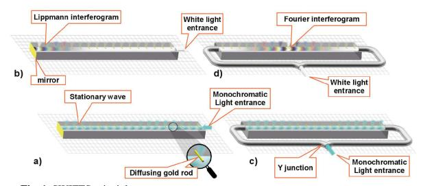
Fig. 1. SWIFTS principles Nanodetectors are placed in the evanescent field of the waveguide. Each detector samples a small part of the flux over a distance smaller than the fringe size. For polychromatic input light, the resulting superimposition of stationary waves lead on to a Fourier interferogram sampled by the set of nanodetectors. The lower 3D artist views present the corresponding SWIFTS devices for colored entrance light and the resulting interferograms.
