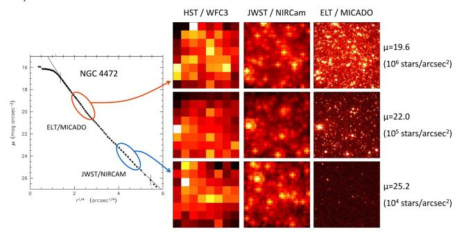
Figure 4. Left: surface brightness of NGC 4472 in the Virgo Cluster, marking the regimes that JWST and MICADO will be able to probe. Right: SimCADO simulations of crowded stellar fields at various surface brightnesses, showing the impact of crowding on what can be measured by HST, JWST, and MICADO.
