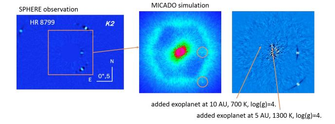
Figure 7. Left: SPHERE image of HR 8799 showing the four known planets.<sup>42</sup> Centre: simulation of 30 s integration with MICADO already reveals the two inner planets.<sup>43</sup> The structure in the image arises from the optical configuration of the telescope and AO system, and its wavefront correction. Right: with basic processing of a series of ADI exposures, one is in principle able to detect other fainter and cooler planets at smaller radii.
