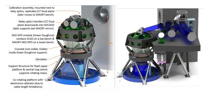
Figure 1. Global MICADO architecture. Left: in 'stand-alone' mode, with the various sub-systems labelled. Right: with MAORY. In the latter configuration, the stand-alone relay optics are replaced by the last fold mirror in the MAORY optical relay; and the calibration unit is moved to the elevator at the ELT telescope focal plane.
