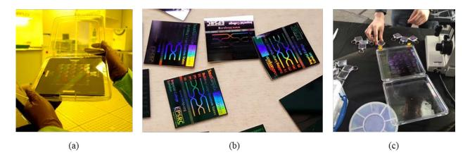
Figure 3. Fabrication and *packaging* of BLOQS chips (a) Chromium mask used for photolithography. (b) Diced chips. The periodic etched grating used in the chip caused light diffraction. (c) Packaging of chips into acrylic snap-in key chains .
