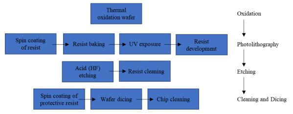
Figure 2. Overview of process flow for chip fabrication.
