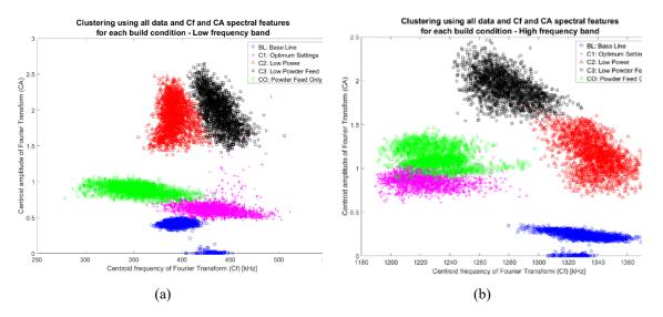
Figure 7. Clustering results for data from a single sensor using centroid frequency (Cf) and centroid amplitude (CA) of spectral data obtained using the Fourier Transform in (a) low frequency and (b) high frequency bands
