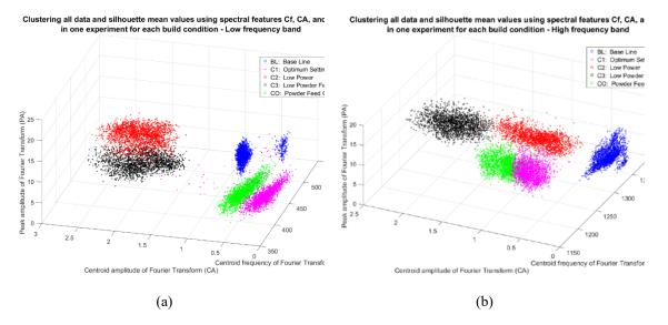
Figure 8. Classification of process conditions using three frequency domain features; peak amplitude of frequency spectrum (*PA*), centroid frequency (*Cf*) and centroid amplitude (*CA*) of spectral data obtained using the Fourier Transform for a single sensor at (a) low frequency and (b) high frequency bands
