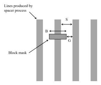
Figure 1. Schematic of block masking for a line-space pattern generated using a spacer process.
