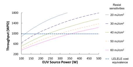
Figure 3. Output per day of a single EUV cluster.<sup>38</sup> This graph was based on assumption of 88% system availability and 75% utilization.
