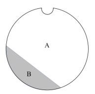
Figure 2. Illustration of non-randomness. For process parameters, such as overlay, values may be within specifications throughout area A of a wafer, while being out of specifications at multiple locations in area B.
