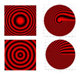
Figure 3. Interferograms of 2-D phase distributions that have linear variation in r. However, in (a) the phase variation is independent of the polar angle, and in (b) the phase distribution also varies linearly with the polar angle.
