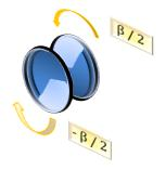
Figure 2. Optical arrangement of two helical phase conjugated masks, for implementing a lens with tunable optical power.
