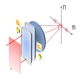
Figure 4. Optical arrangement of two sinusoidal gratings, for controlling diffraction efficiency.
