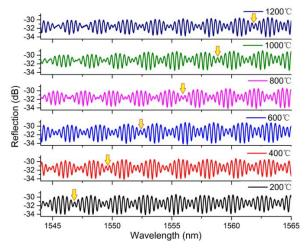
Fig.3.Reflection spectra of proposed sensor under different temperature varying from 200 to 1200°C.
