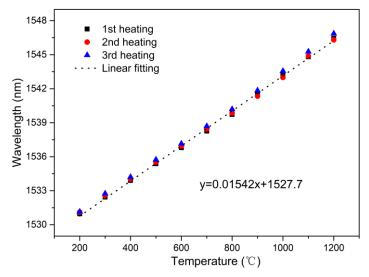
Fig.4. The fitting-figures of the relationship between wavelength drift and temperature variation for HC-PCF based fiber sensor.
