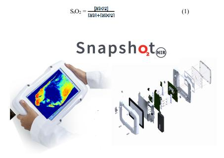
Figure 2. SnapshotNIR is a handheld, battery powered, multispectral imaging system that provides a near real-time measurement of tissue hemoglobin oxygen saturation.
