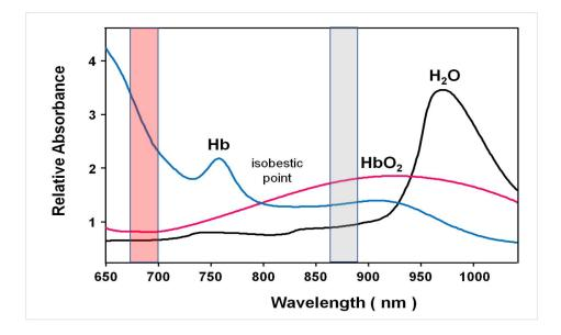
Figure 1. Pulse oximetry measures the reflected or transmitted light from tissue in the deep red and at a longer near-infrared region. The differential light absorption of hemoglobin when carrying oxygen (HbO<sub>2</sub>) and when deoxygenated (Hb) in these two wavelength regions is exploited to determine the relative proportion of HbO<sub>2</sub> to Hb based on the ratio of red to near infrared light that is reflected or transmitted by the tissue.
