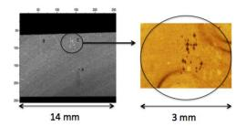
Figure 10: Double crystal X-ray topography, performed at IMEM-CNR, of the ADP sample procured from Saint Gobain (sample size 20 mm × 20 mm × 2 mm). The spots in the area C are dislocations, only present is a very small area of the sample
