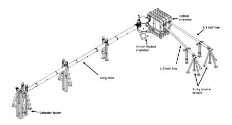
Figure 11: Conceptual design of the BEaTriX vacuum system.
