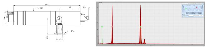
Figure 3: Left: scheme of the Incoatec X-ray microfocus source. Right: measured spectrum of the hybrid X-ray microfocus source with the anode in Ti-Al alloy (50% Al and 50% Ti), showing the X-ray fluorescence lines of both elements (courtesy by Incoatec).
