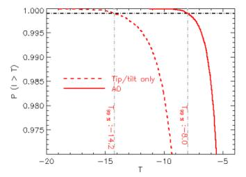
Figure 2. Cumulated fading probability as a function of threshold in dB for a 20 cm aperture system, considering an AO correction of either nr = 1 (tip-tilt) (dashed line) or nr = 3 radial orders (solid line). We indicate the threshold T<sub>99%</sub> corresponding to a 0.999 cumulated probability (hence a 99.9% link availability). This threshold, expressed in dB, is the power loss one has to accept compared to the diffraction limited case.
