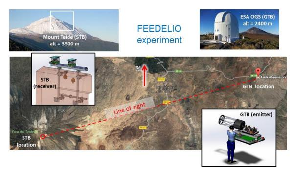
Figure 3.Principle of the FEEDELIO experiment: The Satellite Terminal Breadboard emulates the optical beam coming from a satellite, with an adjustable PAA, and performs signal fluctuations measurements. The Ground Terminal Breadboardemulates an optical ground station equipped with AO pre-compensation of the feeder beam.
