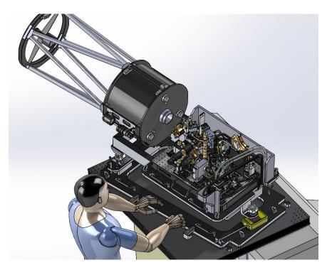
Figure 6. GTB overall design. It is to be settled inside the dome of the OGS of the Teide Observatory.
