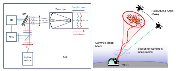
Figure 1. Left : principle of uplink pre-compensation by adaptive optics (AO). Right : The Point Ahead Angle is due to earth rotation. Because of the PAA, the turbulence layer seen by the downlink beam, which is used for wavefront analysis, is not exactly the same as the one seen by the uplink beam, hence limiting the performance of AO precompensation.
