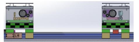
Figure 5.STB design. One module is fixed and aligned with the GTB optical axis ("on-axis module"), the other one ("off-axis module") can be translated through motorization in order to emulate the PAA.
