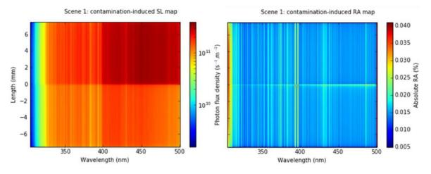
Fig.11 : Resulting stray light irradiance and induced radiometric error in the UVVIS spectrometer due to roughness (top) and contamination (bottom).
