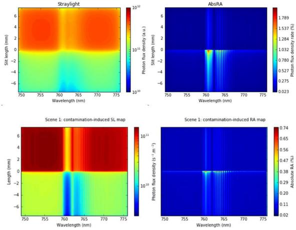
Fig.12 : Resulting stray light irradiance and induced radiometric error in the NIR spectrometer due to roughness (top) and contamination (bottom).
