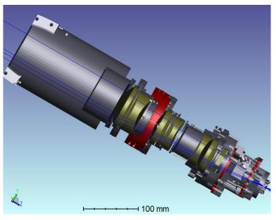
Fig.5 : Cross-section of the non-sequential Zemax telescope model.
