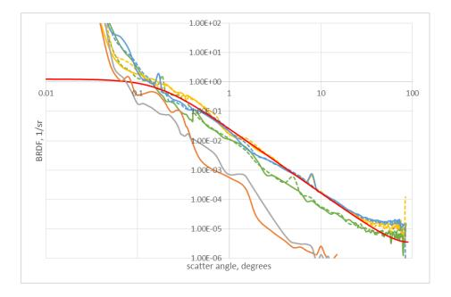
Fig.4 : Example of measured BSDF raw data of several samples with a superimposed a HS model.
