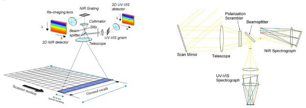
Fig. 2: Sentinel4 instrument measurement principle (left) and Optical design sketch (right).
