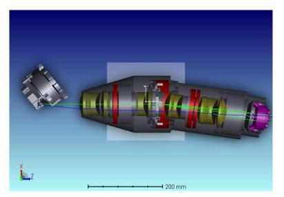
Fig.6 : Cross-section of the non-sequential Zemax UV spectrometer model with the slit assembly on the left.
