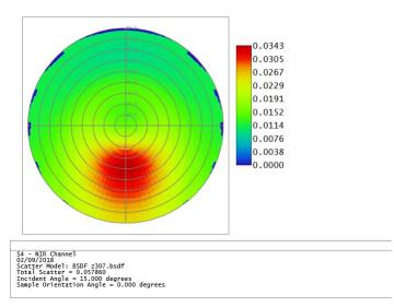
Fig.8 : Z307 BSDF model in Zemax for angle of incidence of 15 degrees. One can see a strong forward scattering.
