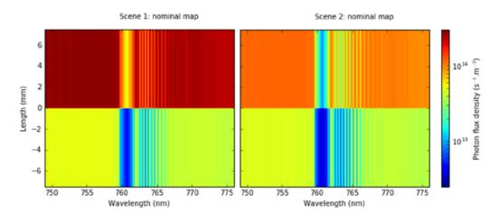
Fig.10 : Reference scenes projected on the NIR spectrometer focal plane.
