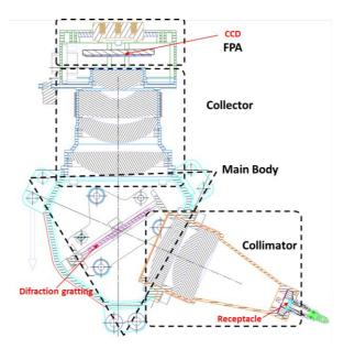
Figure 5. SPU optomechanical layout and "building block"
