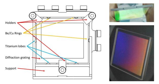
Figure 7. Grating assembly (initial design) and the Volume Phase Holographic Grating (VPHG).
