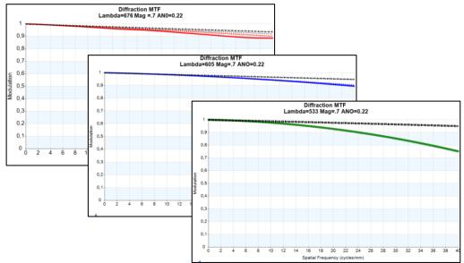
Figure 8. MTF curves for the extreme and central wavelengths in the spectral working range of the spectrometer.
