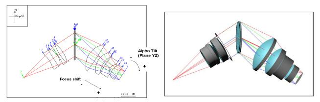
Figure 3. SPU optical ray trace and 3D-design
