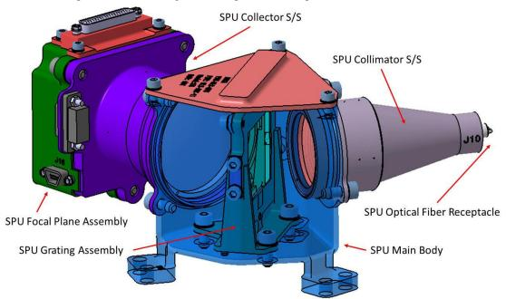
Figure 2. SPU FM Design (main body transparent).
