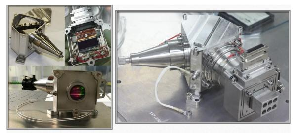
Figure 4. FM Spectrometer Sub-units and whole Unit Titanium structures detailed.
