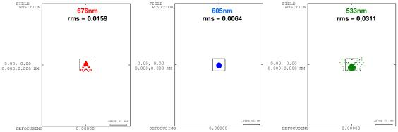
Figure 9. *Spot diagram* for the extreme and central wavelengths in the spectral working range of the SPU. The central box represents the size of a pixel, 15µm.
