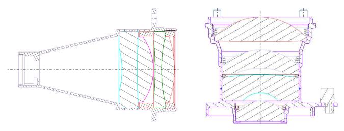
Figure 6. SPU collimator and collector subsystems internal layout
