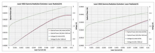
**Figure 6.** (**left**) VCSEL array gamma test results. L-IV curves at 0 and 100 krad for: (left) 3 um aperture VCSEL, (right) 5 um aperture VCSEL
