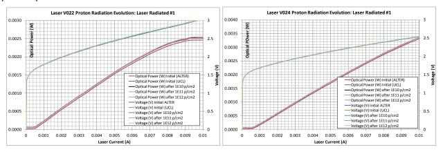
**Figure 7.** (**left**) VCSEL array proton test results. L-IV curves at the three steps for: (left) 3 um aperture VCSEL, (right) 5 um aperture VCSEL
