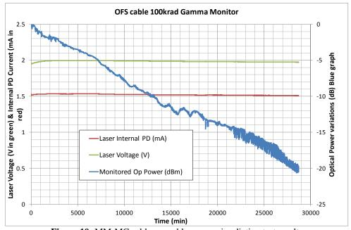
Figure 10: MM-MC cable assembly gamma irradiation test results
