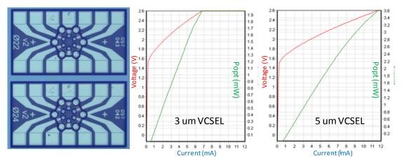
**Figure 1.** (**left**) Microscope image of the 6-channel VCSEL arrays and L-I-V curve of 3 um VCSEL array (**middle**) and 5 um VCSEL (**right**)
