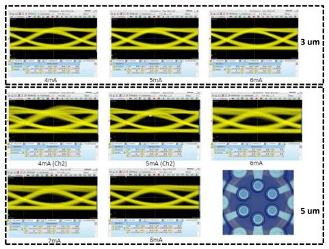
Figure 3. Eye diagrams of VCSEL arrays: (top) 3 um aperture VCSEL, (bottom) 5 um aperture VCSEL. Modulation speed is 25 Gb/s.
