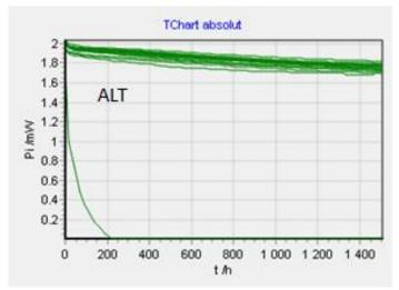
Figure 8: VCSEL array ALT test result
