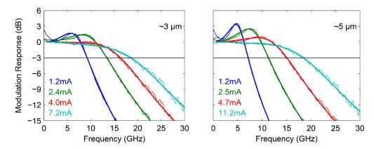
Figure 2. Small signal modulation response at different currents recorded at 25°C: (left) 3 um aperture VCSEL, (right) 5 um aperture VCSEL
