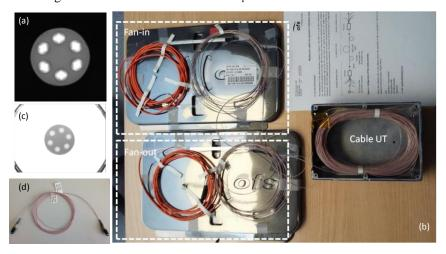
**Figure 9:** a) Profile of multi-mode, multi-core fiber, b) cable sample connected to fan-outs for radiation testing, c) end-face of multi-core MiniAVIM connector and d) assembled multi-core, MiniAVIM patchcord prototype
