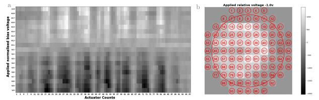
Figure 4: The deformable mirror actuators a) linearity and b) uniformity with respect to the applied bias voltages. The effective surface of the deformable mirror is shown by the red circle.
