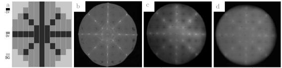
Figure 2: Comparison of deformable mirror response to the a) applied asterisk mask using b) diode laser (635 nm) and a CCD camera c) near infrared thermal source and microbolometer array and d) mid-infrared thermal source and microbolometer array.
