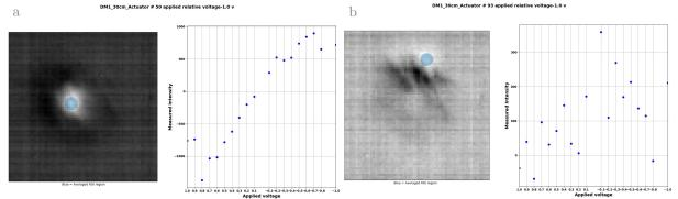
Figure 3: Video 1. Visualisation of spatial variant response of the deformable mirror to the applied bias voltage for a) central actuator and b) marginal actuator. The overlaid blue circle represents the averaged region considered for each measurement on the graph:
