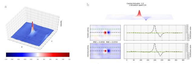
Figure 5: Visualisation of the inter-actuator coupling a) poking the central actuator by -1 bias voltage induces negligible strain on the neighbouring actuators, b) comparison between poking two adjacent actuators in tandem and individually.
