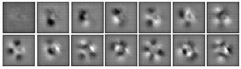
Figure 6: Visualisation of deformable mirror reconstructed far-field eigenmodes. Only 14 modes with largest singular values are shown.
