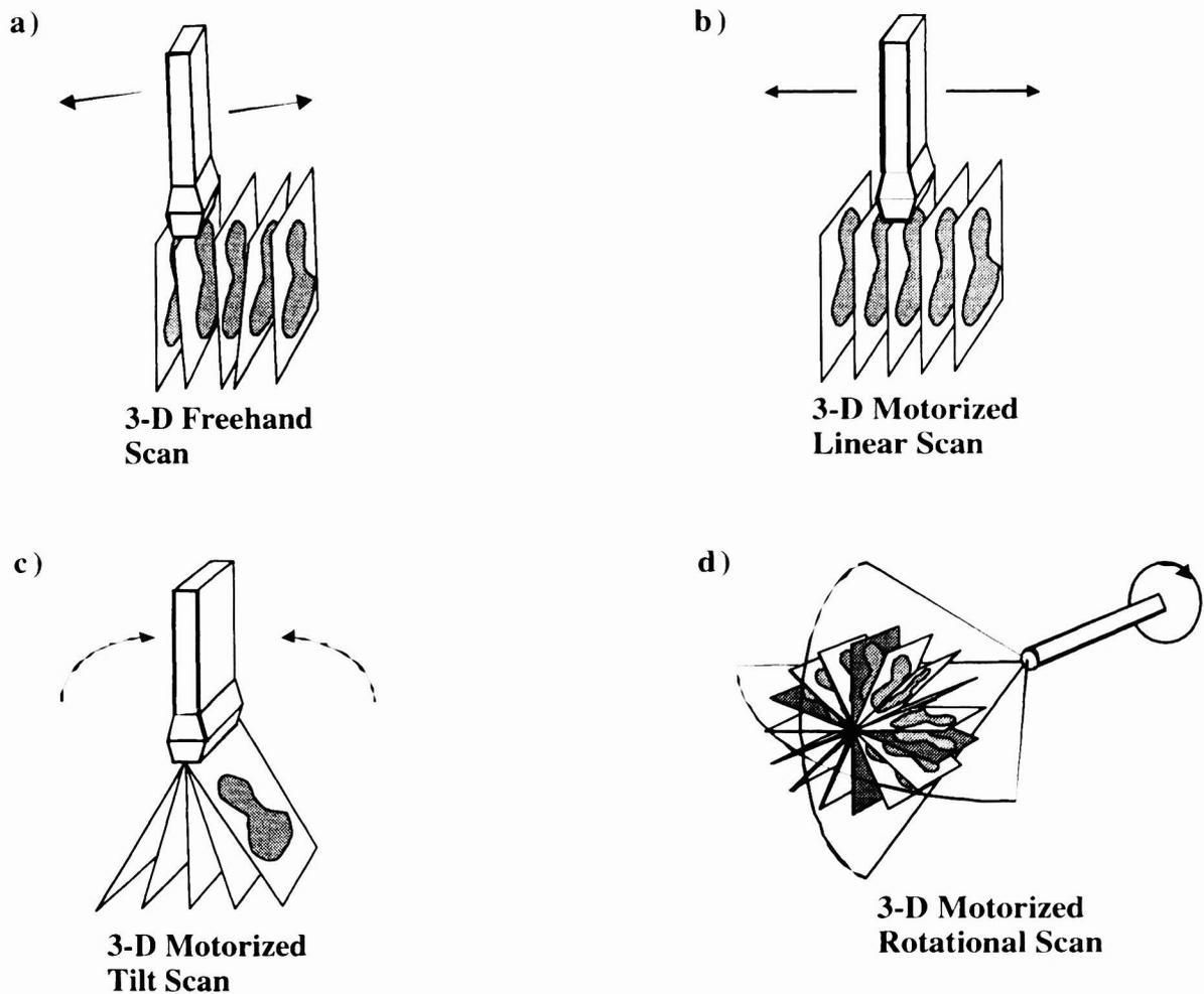
Figure 1. Schematic diagram showing various approaches to 3D ultrasound scanning using conventional ultrasound transducers. a) Free hand scanning with a magnetic positioning device. b) Mechanical scanning with linear motion. c) Mechanical scanning with tilting motion. d) Mechanical scanning with rotational motion.
