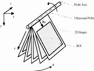
Figure 3. Schematic diagram showing a side-firing transrectal ultrasound transducer being rotated for a 3D imaging scan.
