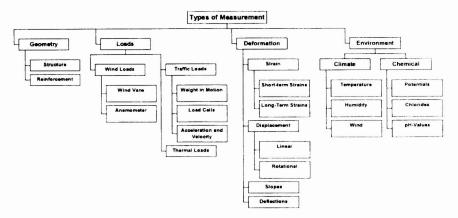
Fig. 1 Hierarchical classification of the different types of measurements
