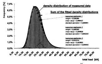
Fig. 17 Real axle load and fitted density functions<sup>10</sup>
