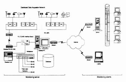
Fig. 13 Instrumentation and communication architecture of the monitoring equipment
