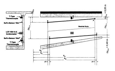
Fig. 9 Instrumented section of a girder box
