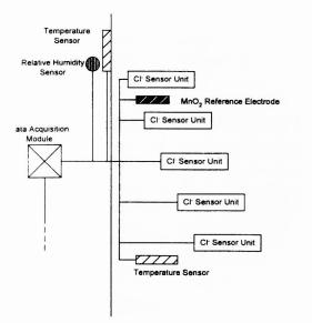
Fig. 12 Corrosion sensor unit<sup>5,6</sup> developed by Zimmermann, Schiegg, Elsener and Böhni
