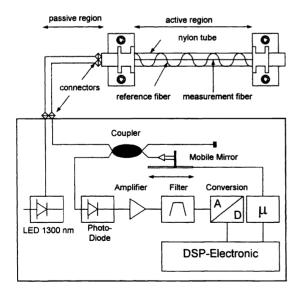
Fig. 5 Low coherence interferometry sensor SOFO<sup>™</sup>, SMARTEC
