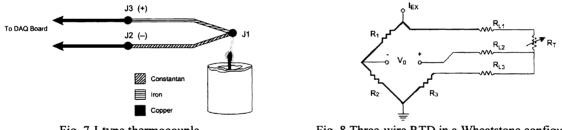
Fig. 7 J-type thermocouple
