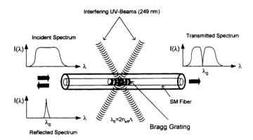
Fig. 4 Bragg Grating fabrication technique and operation principle
