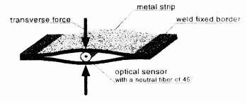
Fig. 10 Fiber optic 'Weight in Motion'- sensor
