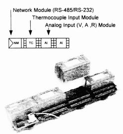
Fig. 14 Distributed data acquisition modules Field Point<sup>™</sup>, National Instruments
