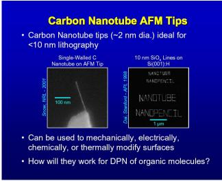
Figure 5. Carbon Nanotubes used as a lithography tool
