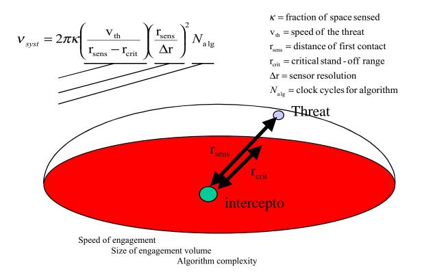
Figure 7. System clock speed requirements in terms of threat engagement speed, search and track volume, and signal processing algorithm complexity.
