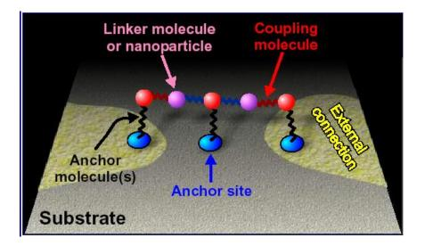
Figure 6. Conceptual view of molecular robes and anchors for bridging the gap between the nanometer and mesoscopic size regimes.
