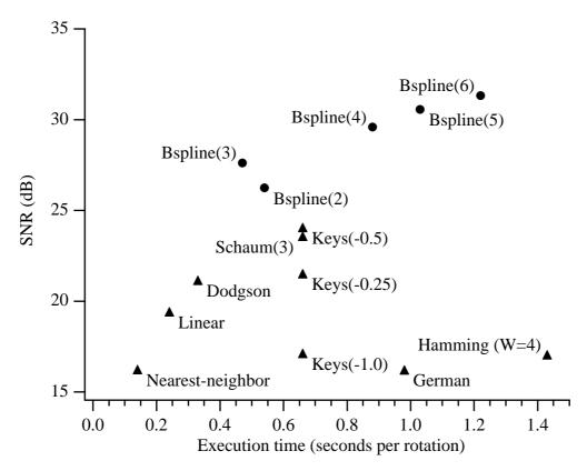
Fig. 1: Cost-performance comparison of various image interpolation algorithm. The experiment involves the application to an image of 15 successive rotation of 24 degrees each.
