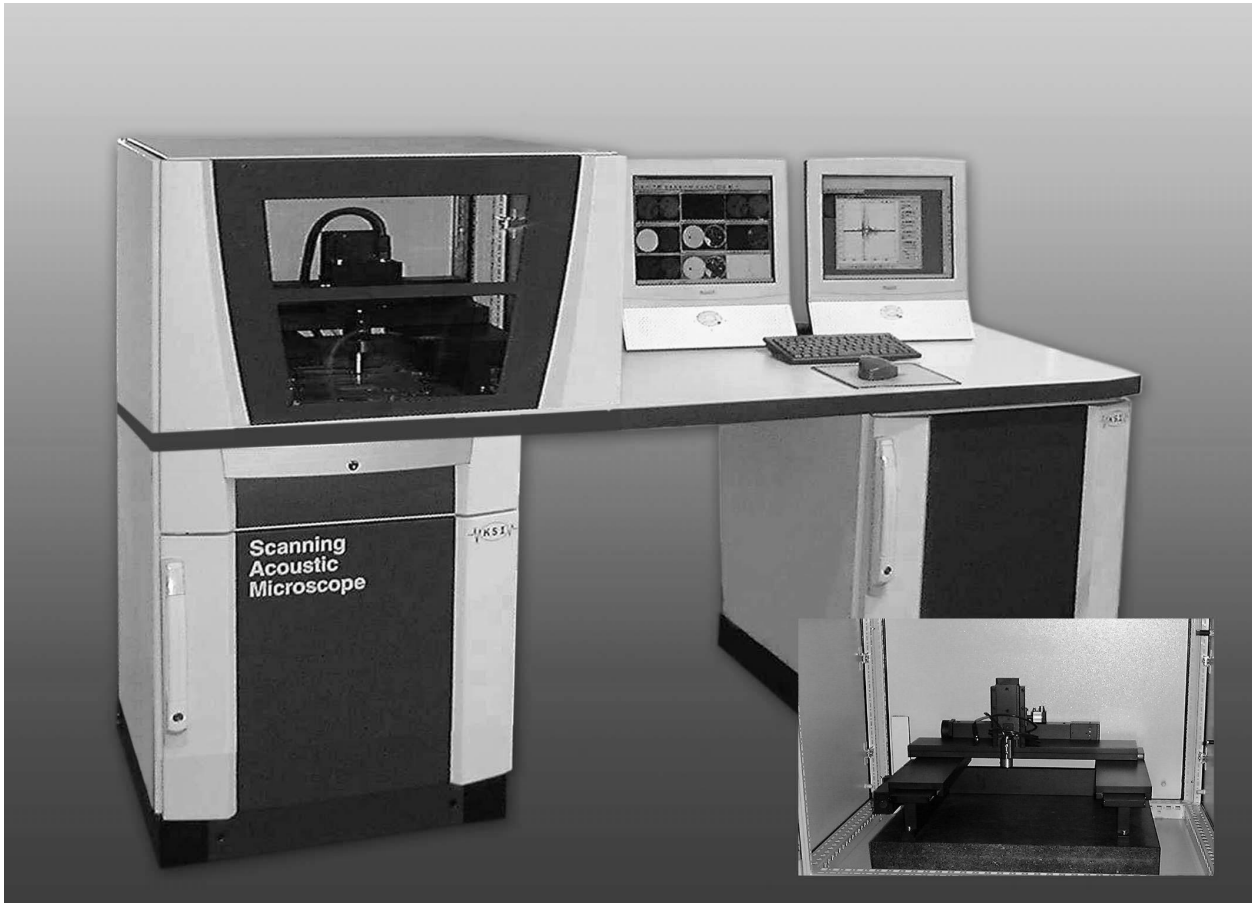
Fig. 1: Acoustic microscope KSI WinSAM Vario III, working in the frequency range from 1 to 400 MHz. It consists out of a high speed high resolution linear scanner system, PC-controlled workstation, and various transducers. The customer can choose the set of transducers and the scanning system individually.
