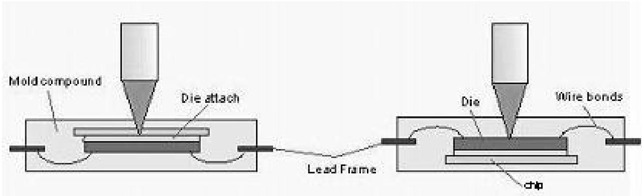
Fig. 3: Ultrasonic inspection of a flip chip is possible from both sides of the sample.
