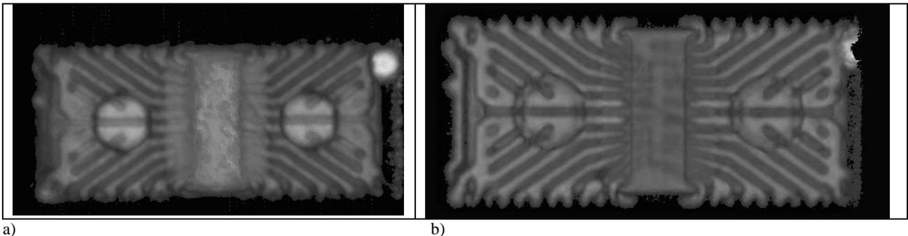
Fig. 4: Comparison between a step motor scanner system (a) and a linear motor scanner system (b) WINSAM Vario III. Due to the smaller step width of the linear motor scanner system and its high precision mechanical linear guide ledge, the resolution in the acoustic image is higher than for the commercial step motor scanning systems. For both images the same transducer (50 MHz center frequency) and the same gate settings were used. The scanning area is  $18.2 \times 8.5 \text{ mm}^2$ .
