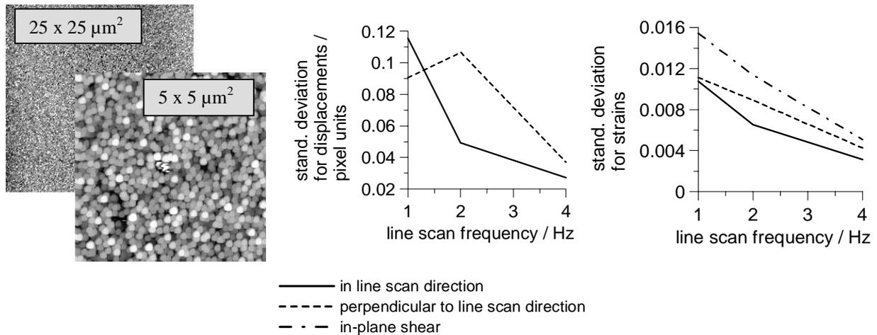
Fig. 4: Estimation of measurement errors for nanoDAC by the help of data standard deviation (over a whole image) determined for subsequently scanned, unaltered samples; non contact scan mode; left side: used Si specimens (sample roughness approx. 10 ... 20 nm); right side: error dependency over the applied line scan frequency
