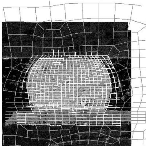
Fig. 3: Deformation measurement at a flip chip solder bump utilizing an ABAQUS finite element mesh, gray mesh: part of the complete undistorted FE mesh, white mesh: deformed FE mesh obtained from a measurement (displacement values 3 times enhanced), base micrographs: SEM images
