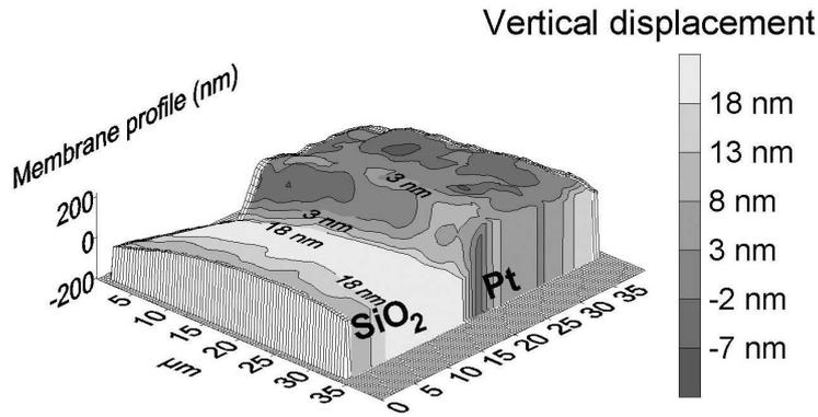
Fig. 12: Residual sensor deformation after heat cycle (SFM based deformation measurement), 3D plot shows part of the membrane layer profile, the coloring (gray scale) indicates the remaining vertical deformation after a heat cycle
