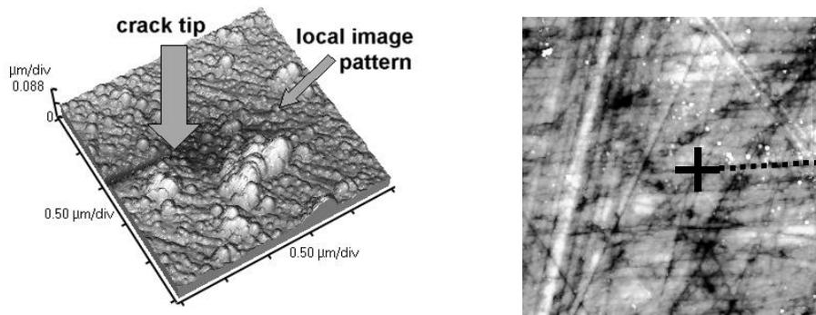
Fig. 7: Examples of typical AFM scans with crack used for nanoDAC analysis, right side: AFM image (size:  $25 \times 25 \mu\text{m}^2$ ) with crack boundary line (.....) and crack tip position determined from the displacement fields (+)
