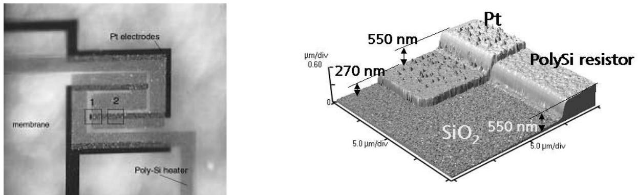
Fig. 10: left side: microscopic image of flow and gas sensor membrane, overall membrane thickness: approx. 2  $\mu\text{m}$ , field of view: approx. 500  $\mu\text{m}$ ; right side: SFM topography scan of gas sensor depicting the Pt layer on top of the  $\text{SiO}_2$  membrane and part of the Poly-Si heater embedded, Source: [14]
