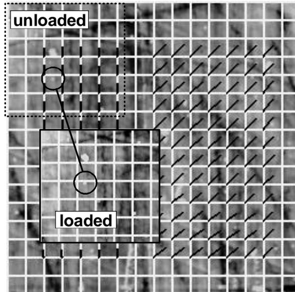
Fig. 2: Principle of displacement field measurement by the comparison of load state images, black arrows: displacement vectors in a regular grid of measurement point (6x enhanced vector size)
