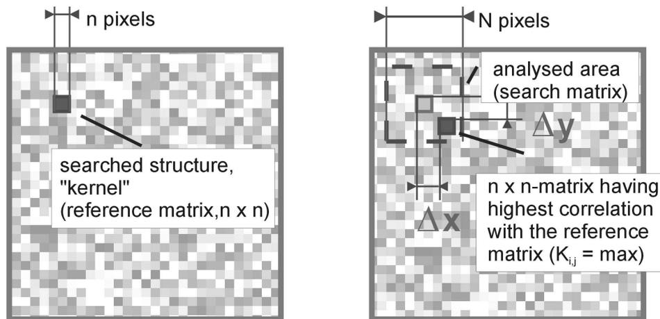
Fig. 1: Displacement evaluation by cross correlation algorithm; (left) reference image at load state 1; (right) image at load state 2 used for comparison
