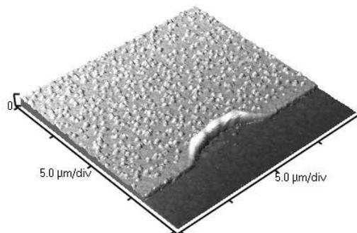
Fig. 11: SFM topography scan of membrane layers after tempering at 450 °C, Pt electrode destruction at edge and corners
