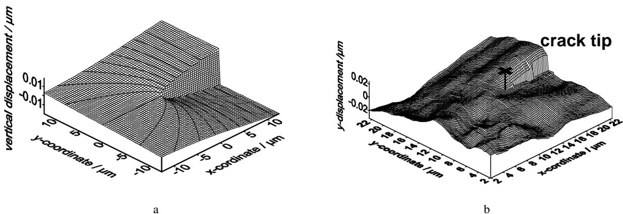
Fig. 8: Displacement measurement from AFM images at the crack tip position, displacement fields  $u_y$  (component perpendicular to the crack boundaries), a – theoretic field from LEFM analytical solution for mode I crack opening, b – measured from AFM topography scans ( $25 \mu\text{m} \times 25 \mu\text{m}$  image size)
