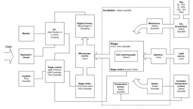
Figure 1. The time-lapse microscopy hardware setup.
