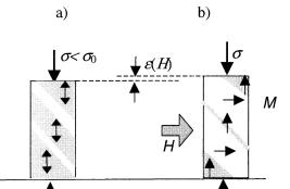
Fig. 2. The shaded and un-shaded regions in panels a) and b) are twin variants with the c axis (c < a) vertical and horizontal, respectively.
