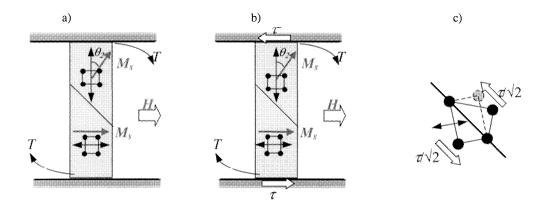
Fig. 4. a) Schematic of twinned Ni-Mn-Ga martensite crystal constrained against the clockwise torque, T, induced by application of a magnetic field. b) The constraint applies a counterclockwise shear couple to the sample to maintain equilibrium. c) Schematic of twinned unit cell straddling the twin boundary. The component of the constraining shear across the twin boundary promotes growth of the field-favored variant.
