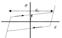
Fig. 1. Schematic stress-strain curve in compression and tension for a typical shape memory material.
