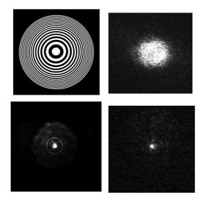
Fig. 7. An example of using OA LC SLM as a pseudo-Fresnel lens. The set of circles (top left) is projected onto LC panel resulting that the collimated beam (top right) is focused to the spot (bottom photographs).
