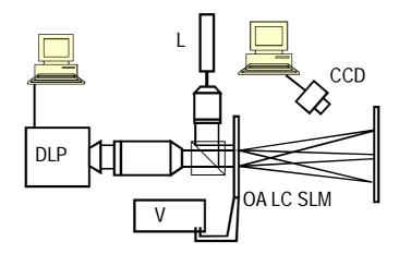
Fig. 4. Digital binary hologram projection system with OA LC SLM. DLP - digital light projector, L -l aser, V - dc voltage supplier, CCD - digital camera.
