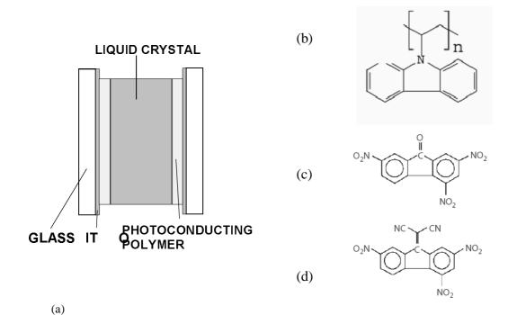
Figure 1. A schematic structure of the liquid crystal panel used in the present studies. The thicknesses of the respective layers are given in the text. The external dc voltage was supplied to the panel with the help of thin wires attached to the ITO conducting layers (a). Chemical formulae of PVK (b), TNF (c) and TNFDM (d).
