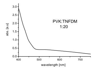
Fig. 2. Absorption spectrum of a PVK:TNFDM thin layer deposited on ITO glass. The charge transfer transition band between carbazole unit and 2,4,7-trinitro-9-fluorenilidene-malononitrile (TNFDM) molecule is visible with maximum around 570 nm.
