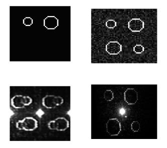
Fig. 5. The diffraction of light on holograms formed in EA (left column) and OA LC SLM's (right column). In the upper row we show an original bitmap and its replica calculated from hologram. Below the hologram reconstructions using EA and OA LC SLM's as the holographic media, respectively are shown.
