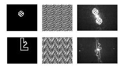
Fig. 6. Examples of bitmaps of 2-D objects (ball and a letter), their computer generated binary holograms that are projected onto OA LC SLM and reconstructed by laser light holograms captured by CCD camera. Besides zero order diffraction the first order spots and images are also seen (cf. reconstructed hologram of L).
