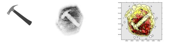
Fig. 3. Example of optical addressing of liquid crystalline panel placed into one arm of Mach-Zehnder interferometer. From left to right are shown: object image superimposed onto 514.5 nm expanded laser beam, phase contrast due to interference of image bearing beam 632.8 nm with reference beam of interferometer and a phase map. The phase difference seen in this case was  $2\pi$  and the phase nonuniformit exceeded  $\pi/4$  mostly due to panel misalignment.
