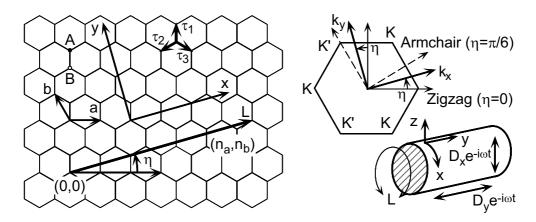
Figure 1. Left: Lattice structure of two-dimensional graphite sheet.  $\eta$  is the chiral angle. The coordinates are chosen in such a way that x is along the circumference of a nanotube and y is along the axis. Right-top: The first Brillouin zone and K and K' points. Right-bottom: The coordinates for a nanotube.
