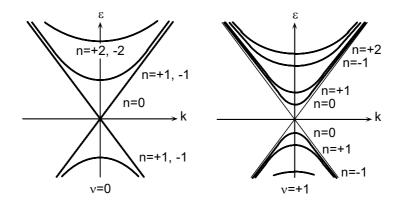
Figure 3. Energy bands of a nanotube obtained in the effective-mass approximation for  $\nu = 0$  (left) and  $\nu = +1$  (right)
