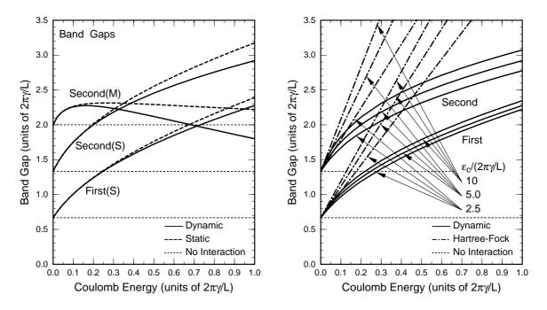
Figure 7. (Left) Calculated gap of a parabolic bands  $(n = \pm 1)$  in a metallic CN (M) and first and second gaps of a semiconducting CN (S) versus the effective strength of the Coulomb interaction.
