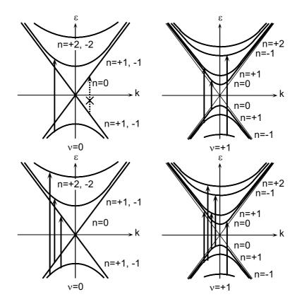
Figure 5. The band structures of a metallic and semiconducting CN. The allowed optical transitions for the parallel polarization are denoted by arrows in the upper figure and those for the perpendicular polarization in the lower figure.
