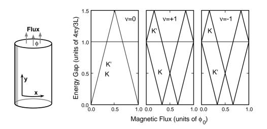
Figure 4. A schematic illustration of magnetic flux passing through a tube cross section (left) and energy gap versus the flux for metallic ( $\nu = 0$ ) and semiconducting ( $\nu = \pm 1$ ) CN (right).
