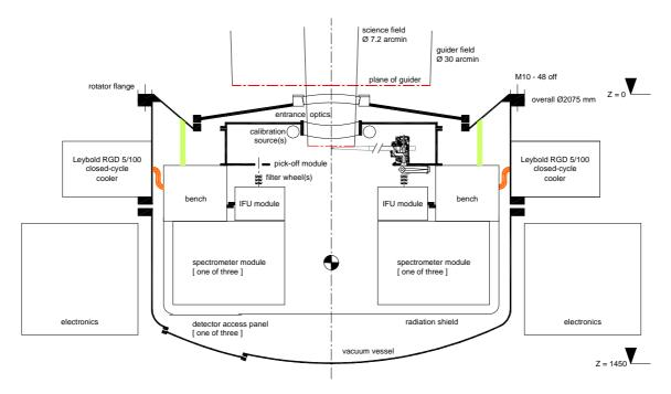
**Figure 4:** Cross-sectional schematic view of KMOS-1 looking down towards the Nasmyth platform. The vacuum vessel is cylindrical with its axis of symmetry aligned with the Nasmyth axis. The electronics racks are supported from the Nasmyth rotator flange by a framework (not shown) which is independent of the vacuum vessel. The annular bench carries all the cooled subsystems and is supported from the rotator flange by a thermally insulated truss structure.
