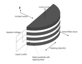
Figure 2. Liquid crystal microwave lens fabricated by Tanaka and Sato<sup>6</sup>.
