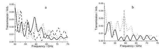
Figure 9. Transmission data as a function of frequency for different voltages applied to all cells. a. The solid line is for no voltage applied, the dotted line is for a voltage of  $1.6 V_{rms}$  and the dashed line is for a voltage of  $3.0 V_{rms}$ . b.The dotted line is for no voltage applied and the solid line is for the top six gaps in each group of ten having applied voltages of  $3.0 V_{rms}$  with the remaining four gaps having applied voltages of  $1.6 V_{rms}$ .
