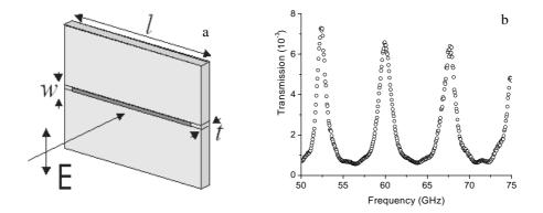
Figure 4. a. Geometry to be explored for resonant transmission of a single variable width slit in an aluminium plate of thickness t. The microwave field is polarised orthogonal to the slit and incident normally on to the metal plate. b. Typical transmissivity scan for a slit width of 250 µm.
