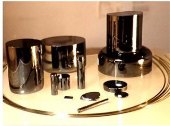
Figure 2 : Bulks of selenide glasses in various sizes photographied with optical fibers.
