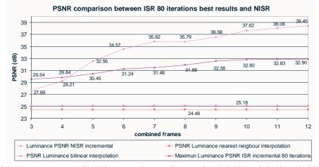
Figure 13: PSNR of the KRANT sequence with 10 incremental output frames using the NISR and the ISR algorithm with 80 iterations.
