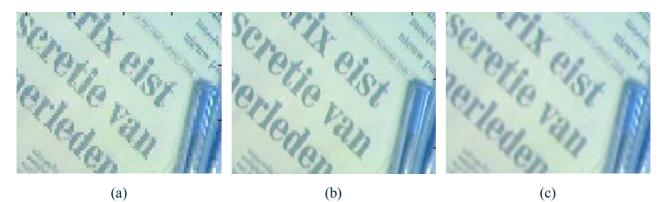
Figure 12: Enlarged detail of the nearest neighbor interpolation of the input image (a), the NISR image combining 12 low-resolution input frames (b) and the bilinear interpolation of the input image (c) for the KRANT sequence.
