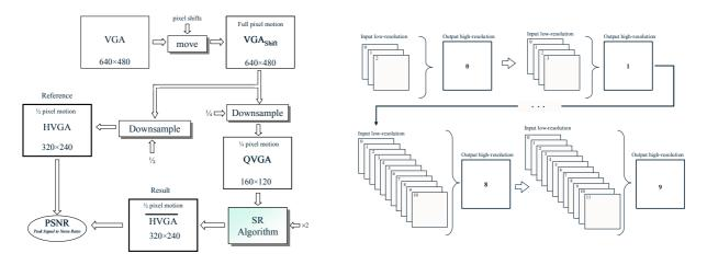
Figure 4: Experimental setup for the test sequences generation.
