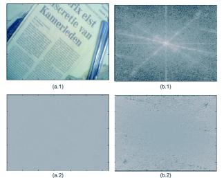
Figure 15: NISR frame after combining 12 low-res frames (a.1) and the magnitude in the frequency domain (b.1) together with their associated errors (a.2 and b.2).
