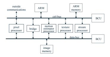
Figure 1: Architecture for the Multi-Standard Video/Image Codec developed by Philips Research.
