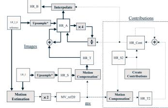
Figure 9: Pseudo-code of the NISR algorithm implemented on the video encoder.
