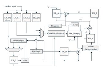
Figure 3: ISR algorithm data flow.
