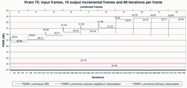
Figure 7: PSNR of the KRANT sequence with 10 incremental output frames using the ISR algorithm with 80 iterations.
