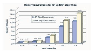
Figure 17: Memory requirements for the ISR and NISR algorithms.
