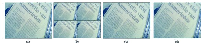
Figure 6: Reference KRANT picture (a), the low-resolution input sequence derived from it (b) and the nearest neighbour (c) and bilinear interpolations (d).
