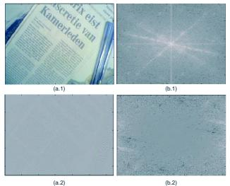
Figure 14: ISR frame after combining 12 low-res frames (a.1) and the magnitude in the frequency domain (b.1) together with their associated errors (a.2 and b.2).
