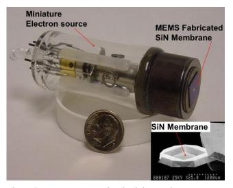
Figure 2. Vacuum encapsulated miniature electron source. The encapsulation membrane is anodically bonded to the electron source. Inset shows the MEMS-fabricated 200nm-thick SiN membrane.
