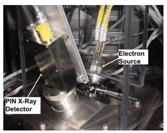
Figure 3. View of the top flange of the environmental chamber showing the electron source and the solid-state, PIN diode, x-ray fluorescence detector. The composition and pressure of gaseous mixtures within the environmental chamber can be adjusted to simulate planetary atmospheric conditions.
