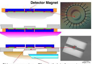
Si beam resonator Fiber optic interferometer
