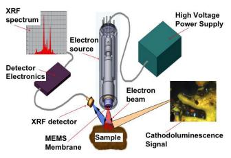
Figure 1: Schematic diagram showing the main components and the operation of the ELXS instrument. A high energy (20 keV) electron beam is generated within the vacuum-encapsulated electron source. The beam traverses the MEMS-fabricated, SiN encapsulation membrane and strikes the sample generating x-ray fluorescence and optical luminescence (cathodoluminescence).
