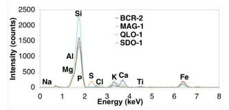
Figure 5. ELXS x-ray fluorescence spectra obtained at Martian environmental pressure from four mineral samples described in the text. Each mineral is easily identified from characteristic peaks present in its respective XRF spectrum. Elemental compositions for elements with atomic number greater than 11 (x-ray detector cutoff) closely match the USGS certified values.
