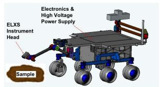
Figure 8. Artist's conception showing the deployment scenario for the ELXS instrument integrated on a planetary exploration rover. The ELXS instrument head is mounted on the rover arm while the control electronics is located within the "Warm Electronics Box" of the rover.
