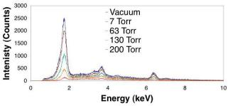
Figure 6. Attenuation of the electron-beam excited XRF signal with increase in ambient pressure. The XRF spectrum was acquired from a Basalt sample. A 7 Torr pressure (Martian ambient) shows negligible attennuation while an ambient pressure over 100 Torr shows significant XRF signal attenuation. The attenuation is more pronounced at lower x-ray energies.
