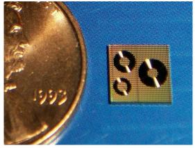
Figure 11 High index long waveguide spirals with lengths 0.5, 1.0 and 1.5 meters.
