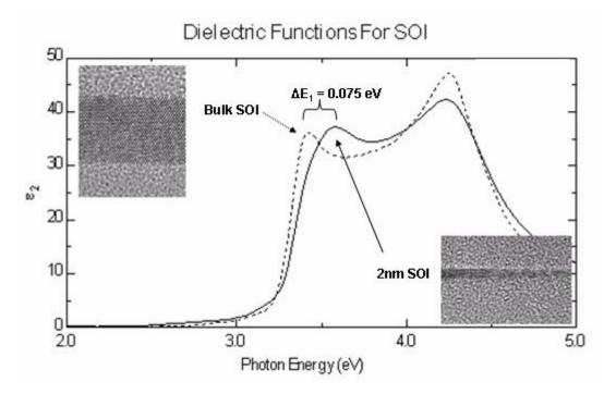
Figure 2. The shift in the E1 critical point of silicon is shown for a 2 nm thick SOI film.
