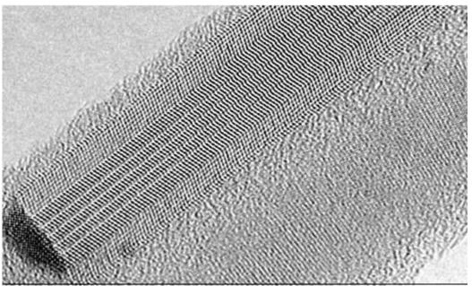
Figure 3. Silicon Nanowire grown for Korgel Group and imaged by Alex Thesen. Figure courtesy Alex Thesen of Zeiss.
